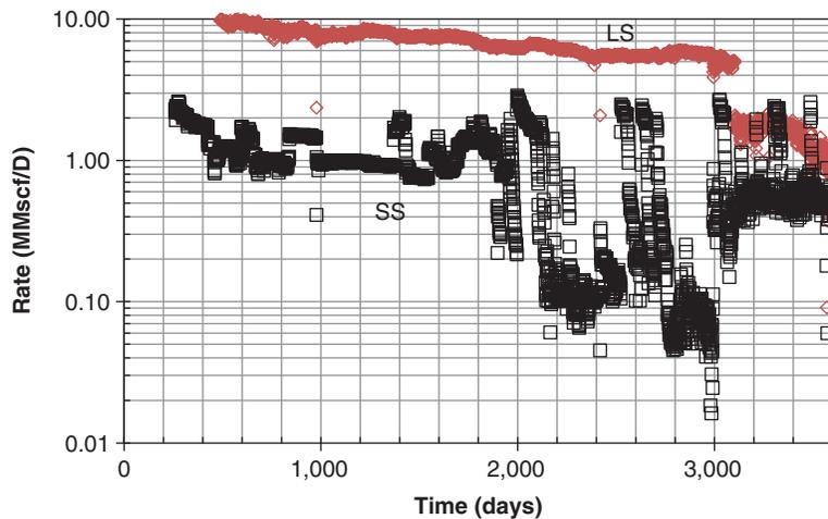
**Fig. P1.3.2—Notice the long string (LS) produced at a much higher rate than the short string (SS). Decline rate for the deeper well,  $D = 5\%/yr$ . The short string experienced sanding problems over much of its producing life. Well problems caused erratic production rates after approximately 1,900 days.**
