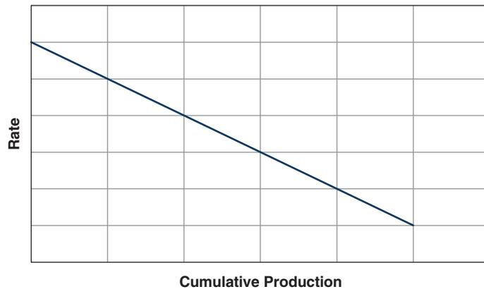
Fig. 1.7—A straight line plot for a rate vs. time curve represents an exponential decline.
