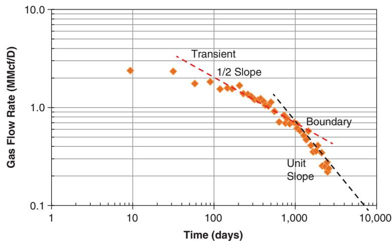
**Fig. 1.9**—The log rate- log time plot divides well performance history into transient and boundary-dominated depletion regimes. This plot is particularly important when studying low-permeability wells.
