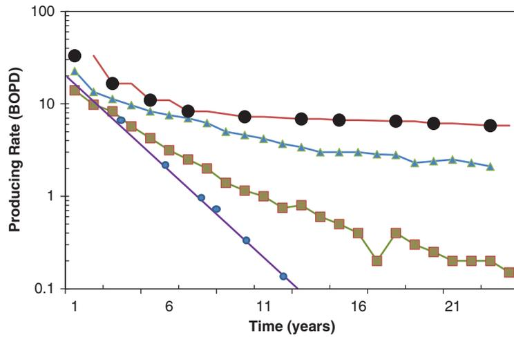
Fig. 1.3—Definitive shapes defined by the Arps equation. It can be observed that the top two curves never decline to a zero production rate, indicating transient flow conditions possible because of commingled layers (no crossflow) and Arps should be applied with caution. Decline curves are normally presented on a semilog rate vs. time plot.
