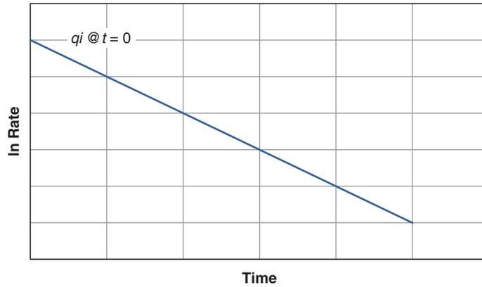
Fig. 1.6—The well-known exponential logarithmic rate vs. time plot which is the usual initial plot for all decline curve analysis. Predict future performance by extrapolating along the straight line. Note value of  $q_i$  at  $t = 0$ .
