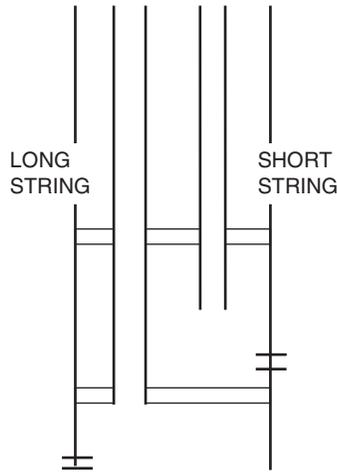
**Fig. P1.3.1—Completion setup of a dually completed gas well.**
