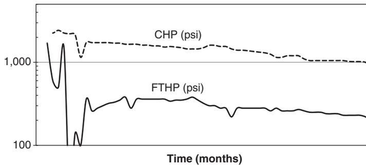
Fig. P1.5.1—A north Texas gas/condensate well. CHP = Casinghead pressure.
