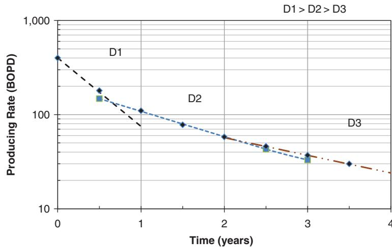
Fig. 1.4—Divide a curved semilog rate vs. time plot into a series of chords of decreasing slope. The declining straight-line slopes form a smoothly declining curve in the case for Fig. 1.2.
