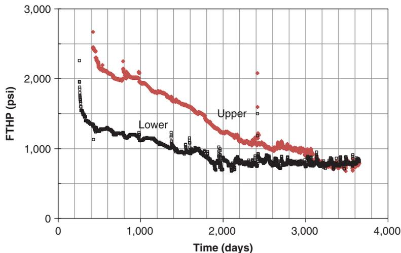
**Fig. P1.3.3—Flowing-tubinghead-pressure history for the two completions.**
