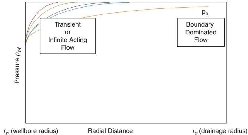
**Fig. 1.1—Differentiating between constantly expanding (transient) and constant-volume (boundary dominated) conditions. An expanding drainage radius indicates an increasing reservoir volume. The pressure drop between ( $r_w$ ) and ( $r_e$ ) must begin to decline because a closed outer boundary has been encountered at boundary dominated conditions.**
