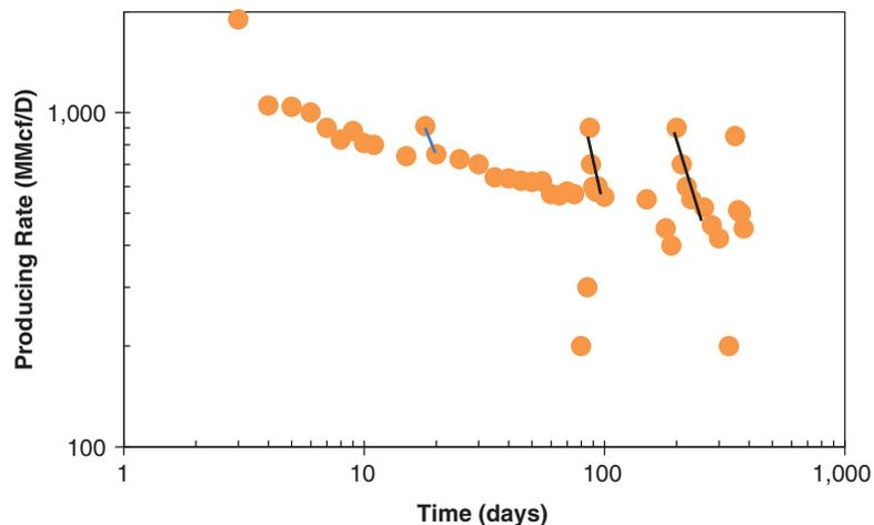
**Fig. 1.10**—Depletion history for the North Sea field. In each instance production soon declined to the field depletion rate after being reopened to flow. Adapted from Fetkovich (1980).
