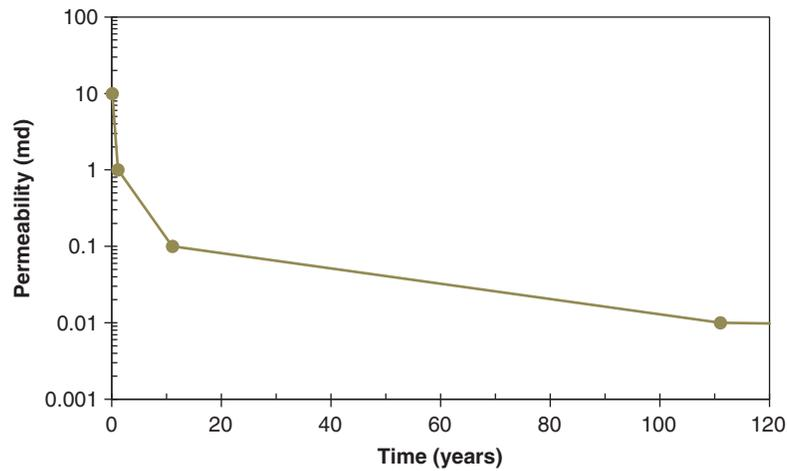
**Fig. 1.2**—Transient conditions can last for an extraordinarily long time for the very-low-permeability gas case.
