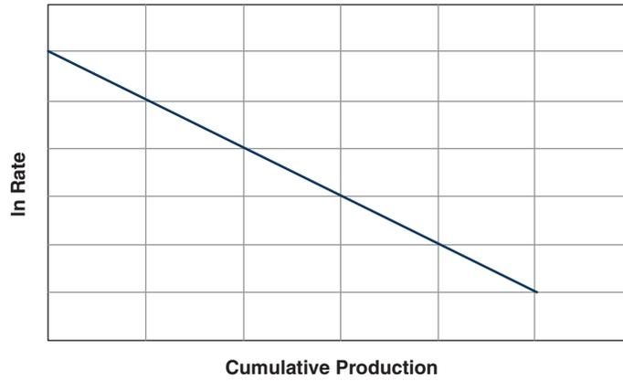
Fig. 1.8—A straight line results when the cumulative recovery equation is rearranged in the form of a straight line.
