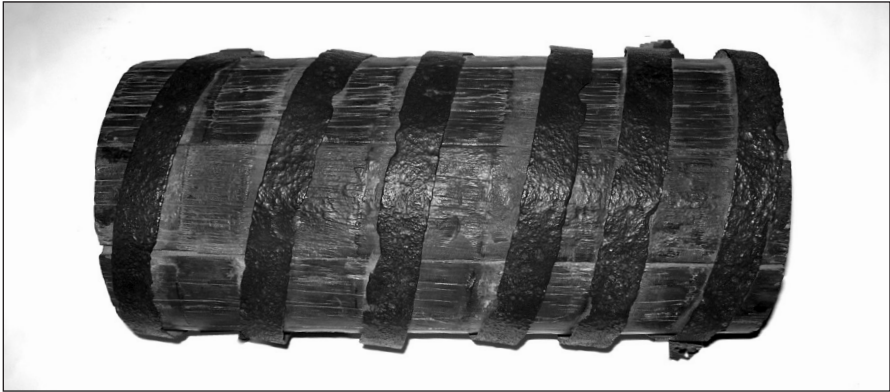
Fig. 2-5. Hollowed-out log used to transport gas. Note the iron bands added to reinforce the wood.
