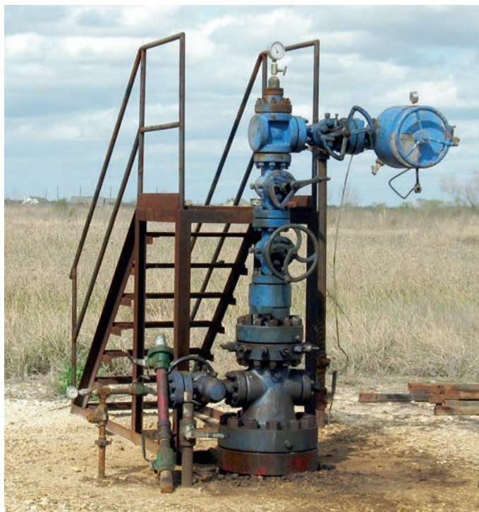
Fig. 6—2. Natural gas wellhead. Often called a Christmas tree or just tree, it is located atop a well. Production field workers adjust the various valves and gauges on it to control pressures and flows.
