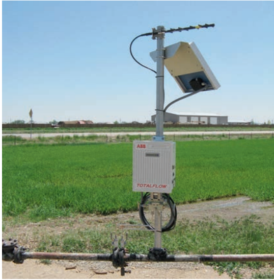
Fig. 6–3. Orifice meter. The meter at the production processing area is typically the first component in the natural gas gathering system.
