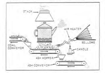
As you see, it is becoming more complicated. Now, we have a chimney or stack to remove the gas of combustion and a heater to heat the air from the bellows before it is blown into the furnace. Also, we have put in an ash conveyor.
