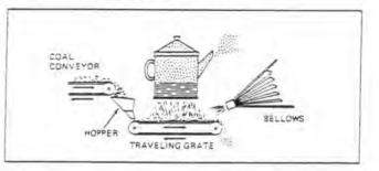
Here, we see a belt conveyor transporting coal to the furnace where it is burned on a traveling grate stoker. Air for combustion is supplied by a bellows.
